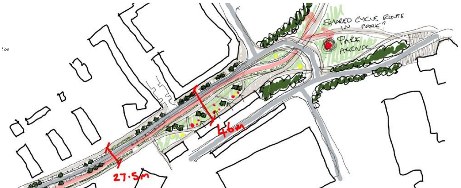
Generally Beach Boulevard is approximately 27.5m wide (measured from back of pavement on either side) however as Beach Boulevard reaches the Queens Links there is an opportunity for this to widen to approximately 46m. This could bring additional design flexibility to this section of the Boulevard and allow the character of the new Park to extend back towards the City.
